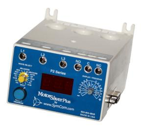
SymCom's Model 777-HVR-LR-P2 is a fully programmable electronic overload relay. It is designed to monitor and protect any 3-phase, 340-480VAC motor drawing 1-800 full load amps (external CTs are required above 9 amps). This unit's Form C contacts are pilot duty rated at 470VA @ 600VAC for applications where a control power transformer (CPT) is not used on a 480V system. The unit provides unsurpassed protection from faulty voltage, underload and overload conditions.
